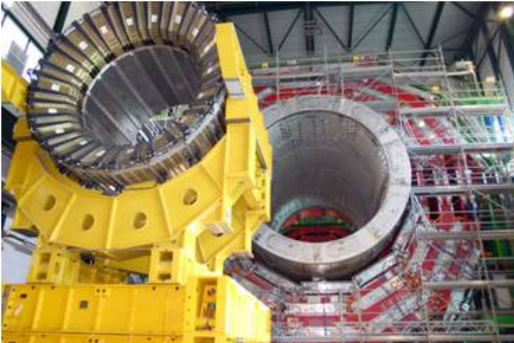
Superconducting solenoid, a part of the detector CMS within the LHC (Large Hadron Collider) at CERN http://en.wikipedia.org/wiki/Image:HCAL_Prepared_for_insertion.jpg
