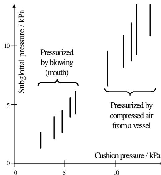
Figure 2: Main results of the experiments of Wethlo. The lines indicate the ranges of subglottal pressure in which voicing occurred for a given cushion pressure (after Wethlo 1913).
