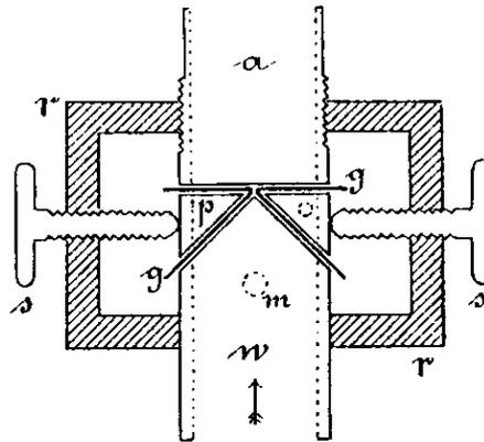
Figure 1: Cross section of the cushion pipe (from the original publication of Wethlo 1913).
