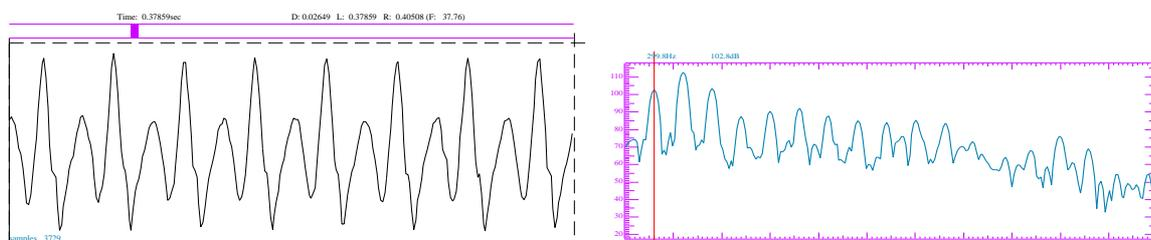
*Figure 5: Waveform and spectrum of the signal produced by the large cushion pipe according to the conditions described in Table 2. Frequency range of the spectrum: (0 ... 5.5) kHz.*
