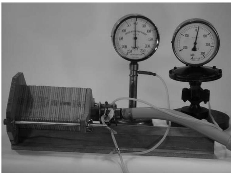
*Figure 6: The experimental setup consisting of the wooden vocal tract model and the large cushion pipe.*
