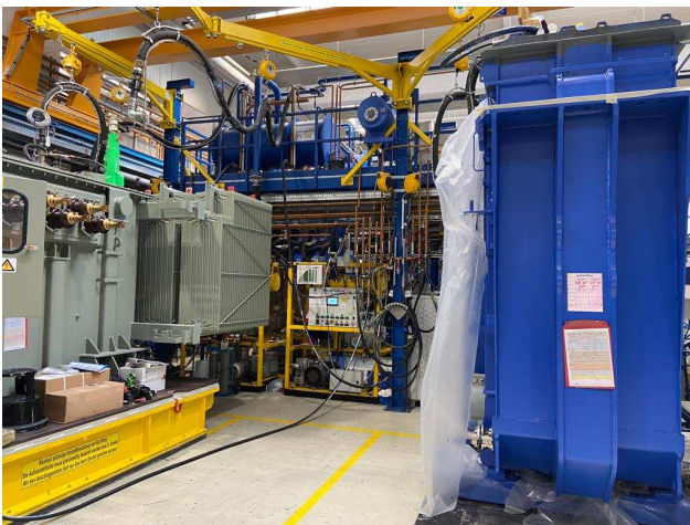
Fig. 2. External filling system for filling processes
