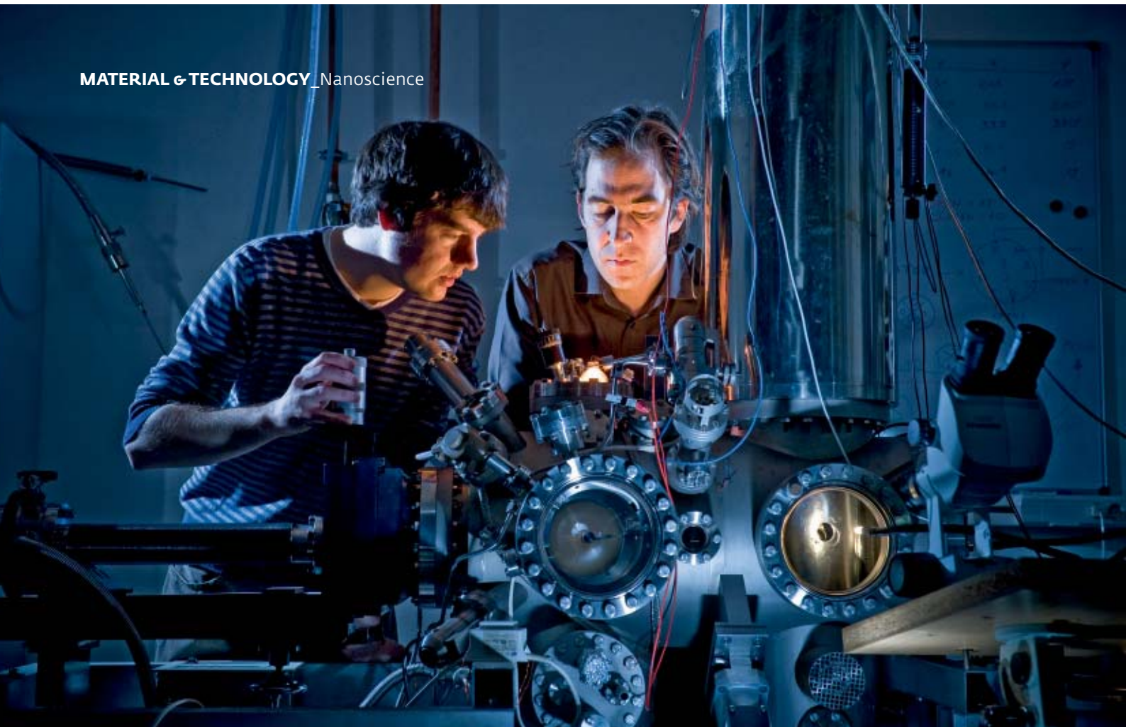
A machine that Leonhard Grill (right) and his team use to study nanomachines: Together with Alex Saywell, he transfers a sample from the preparation chamber to the measuring position in the ultra-high-vacuum system. There, the researchers inspect the sample with, for example, a scanning tunneling microscope. The great cylinder in the right half of the image contains the cryostats that are used to cool the sample.
