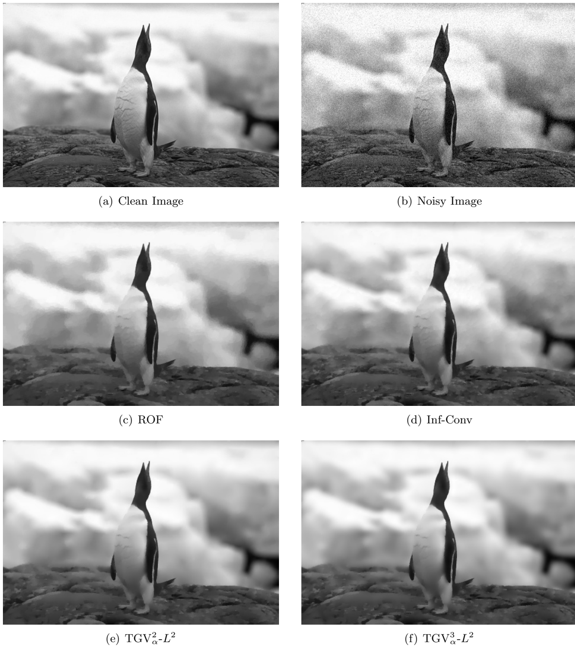
Figure 7. Denoising of a natural image (a). (b) shows the 481 \times 321 noisy input image containing zero mean Gaussian noise with standard deviation \sigma = 0.05 . (c)–(f) show the results of ROF, Inf-Conv, TGV_{\alpha}^2-L^2 , and TGV_{\alpha}^3-L^2 image denoising (see also Figure 8).
