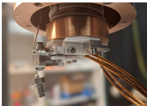
Figure 1: A combined field emission and gas field ionization source
