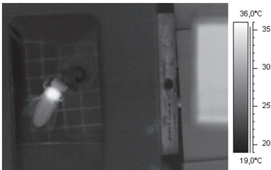
Fig. 1: Infrared thermogram of a honeybee forager sucking 0.5 M sucrose from an artificial flower inside the respirometric chamber. Surface temperatures are 35.6 °C for the thorax, ~26.7 °C for the head, and ~25.7 °C for the abdomen. T_a (chamber) = 20 °C. Radiation < 100 W/m 2 . Right hand rectangle shows Peltier-driven reference source for infrared camera calibration.
