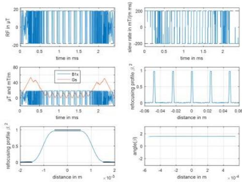
Figure 1: Time-optimal RF and slice selective gradient shapes and Bloch simulations
