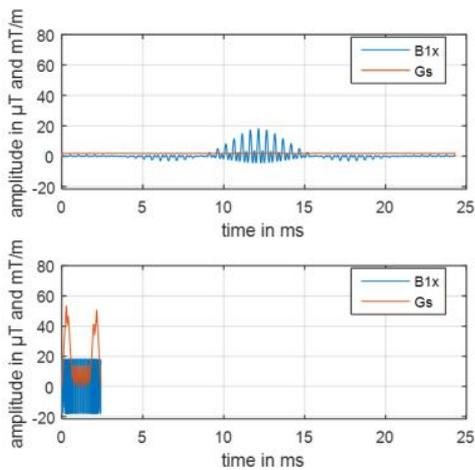
Figure 2: Comparison of the overall pulse duration of a conventional SMS pulse using superposition (top) vs the time-optimal pulse and gradient pair shown in Figure 1 (bottom)
