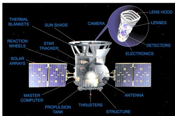
Fig 1: Transiting Exoplanets Survey Satellite Overview [2]
