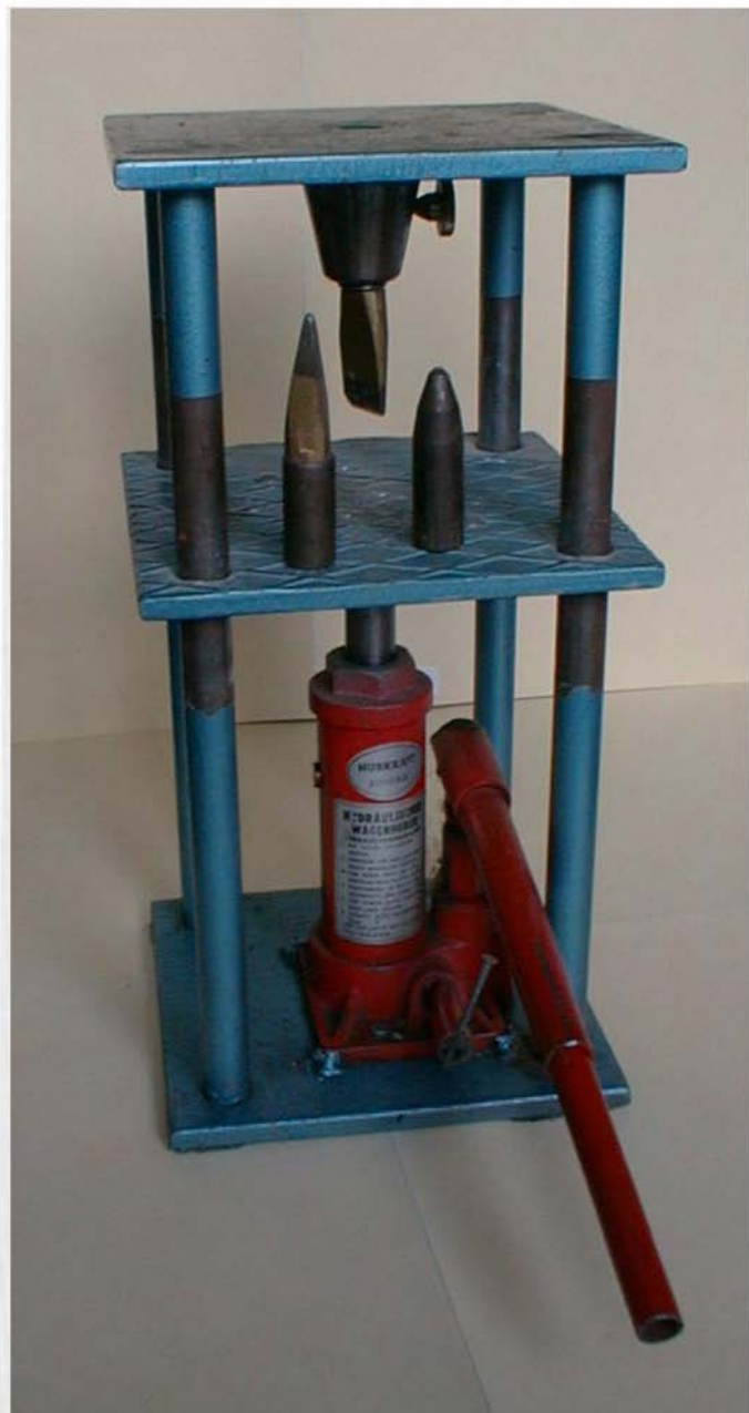
Fig. 1. Home-made "rock-hacker" with interchangeable chisels and using a typical car "jack".
