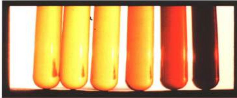
ZSIGMONDY-Ag- COLLOIDS: Mean sizes increasing from 6 to 60 nm Top: Transmitted light. Bottom: Scattered light
