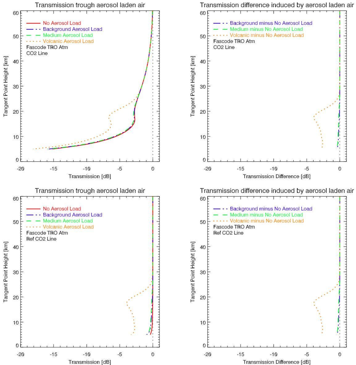
**Figure 4.4:** Propagation modeling results for the ACCURATE CO<sub>2</sub> absorption (upper row) and reference (lower row) channels in air with no (red, solid), background (blue, dashed-dotted), medium (green, dashed), and volcanic (orange, dotted) aerosol load, respectively. The left panels show direct transmission results and the right ones the difference between the transmissions of aerosol laden air vs. clear air.
