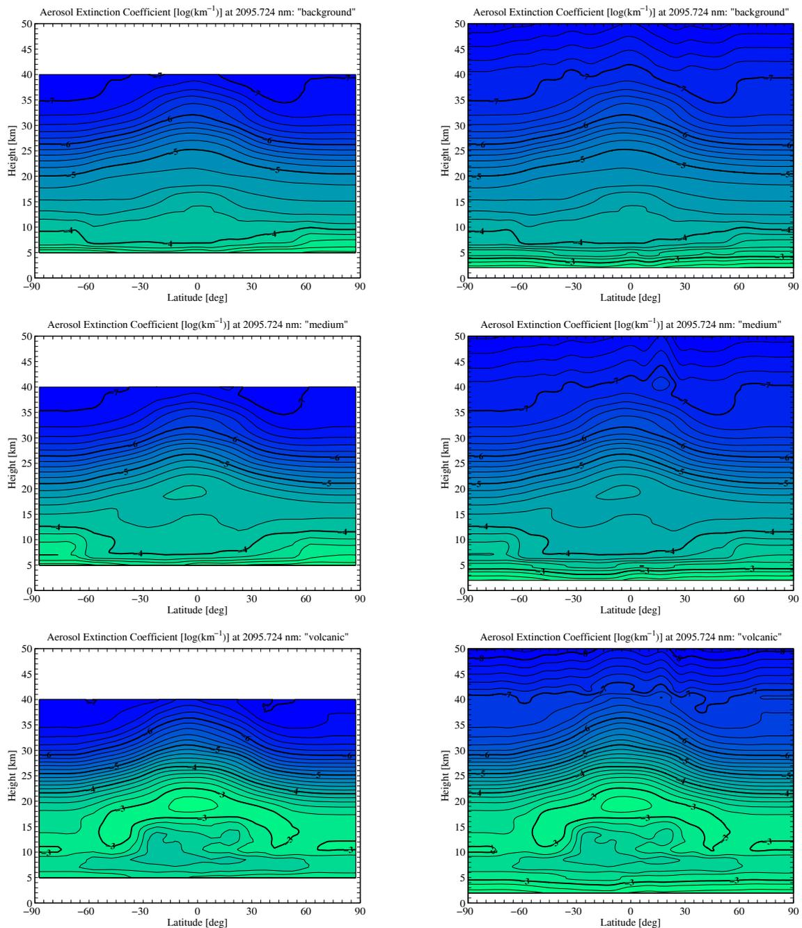
**Figure 4.3:** Overview on aerosol extinction coefficient model fields at the ACCURATE CO<sub>2</sub> line center frequency near 2.1 μm both at the native grid (left column; same 5° x 0.5 km grid as for the basic tables presented in the previous subsection) and a fine interpolated grid (right column; 0.5° x 0.05 km grid extending from 2 km to 50 km height). The rows show the three cases of “background” (top), “medium” (middle), and “volcanic” (bottom) aerosol load, respectively.
