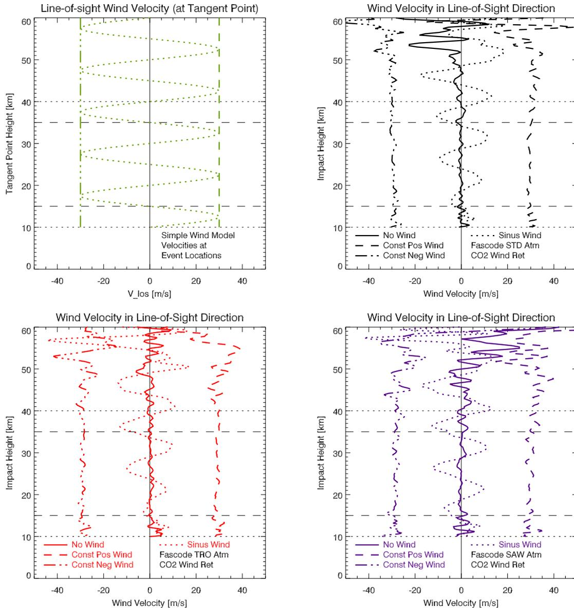
**Figure 4.10:** Initial wind retrieval results: retrieved wind velocities for the same occultation events and atmosphere and wind conditions as shown in Figure 4.6. The upper left panel shows the “true” wind velocities at occultation event location underlying the SWIR propagation modeling; the other three panels show the retrieval results.
