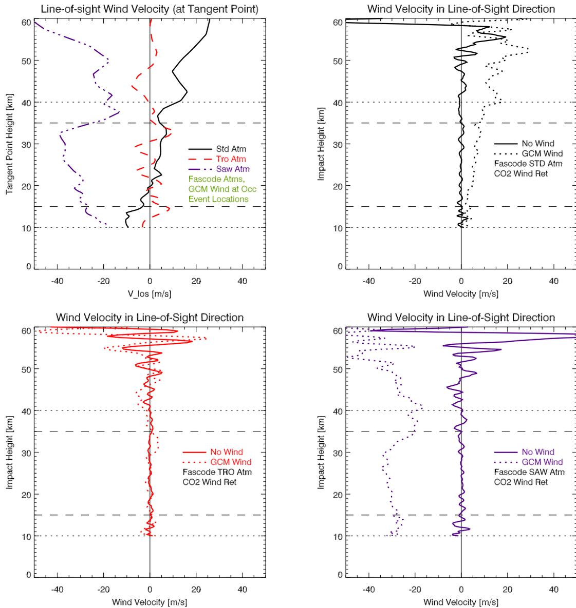
**Figure 4.11:** Initial wind retrieval results: retrieved wind velocities for the same occultation events and atmosphere and wind conditions as shown in Figure 4.7. The upper left panel shows the “true” wind velocities at occultation event location underlying the SWIR propagation modeling; the other three panels show the retrieval results.
