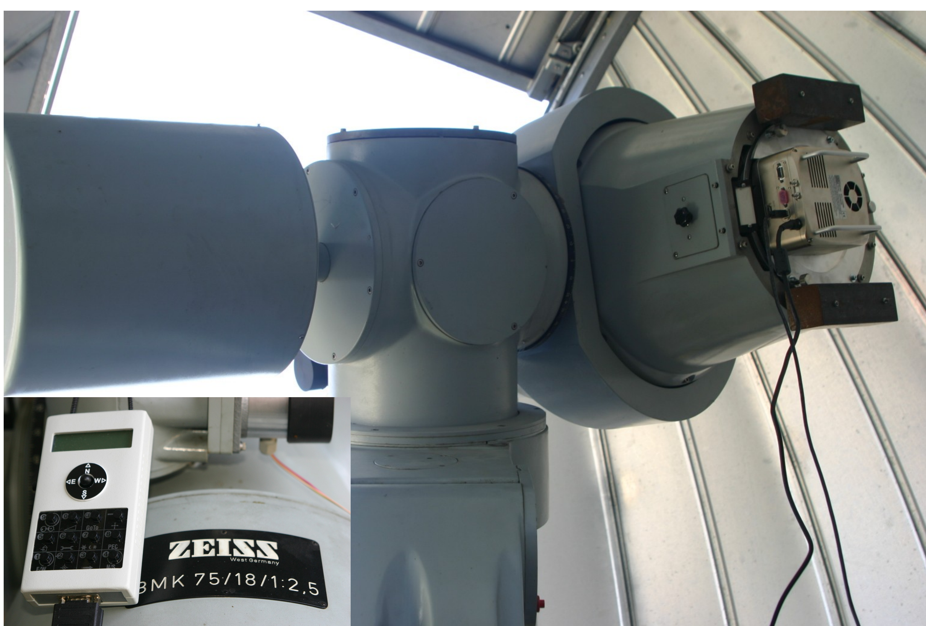
Figure 1. Zeiss BMK 75/18/1:2,5 with SBIG STL-11000M; insert: Pulsar Commander hand control box.
